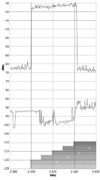
Fig. 2. Wireless transmission at Netatmo NSC01-EU
